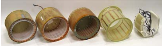
Figure 1: Photograph of the 5 coils. Left to right: TEM small , TEM large , High-Pass Birdcage (HPBC), Hybrid Birdcage (Hybrid BC), 8 channel receive array.
