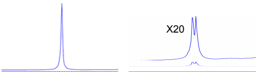
Figure 3. Proton spectra of rat femur bone specimen. Left: non-suppression one pulse ( 8 \mu\text{s} ) spectrum; Right: water and fat suppressed proton spectrum, in which the full width of the observed resonance at half height was \sim 1.2 \text{ kHz} .
