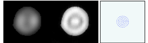
Fig2. Simulated results for spiral spokes placement (right), in-plane modulation (left), and corrected profile (center)
