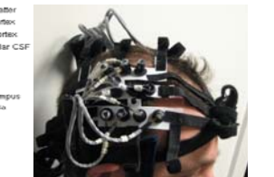
Figure 8. Approximate placement of NIRS probes on the subject's right side (symmetrical probes on the left). The 4 optodes in the center strip are sources, the 8 optodes in the side strips are detectors. Each source emits two wavelengths. The NIRS waveforms are derived from 27 source-detector combinations.
