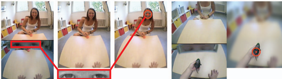
Figure 2. Eye-Tracking process. 1 st column: the location of the eyes in the image is extracted automatically during post-hoc calibration. 2 nd column: the direction of gaze is computed automatically from the eyes image through support vector regression. 3 rd column: to highlight the direction of central vision (indicated by a crosshair), the image is blurred except for an area of 10 degrees radius around the center of the gaze. 4 th & 5 th columns Gaze tracking example while looking downwards: the system uses the whole eye region (shading of the eyelids, shape of the eyelashes, etc) to compute the gaze direction. doi:10.1371/journal.pone.0044144.g002
