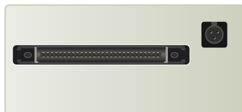
Figure 2-12. ExG AUX Box (side view), connection for ribbon cable (left) and "PWR" input for the power supply (right)
