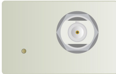
Figure 2-22. SyncBox Scanner Interface (side view), yellow "PWR" LED (left) and "Input" port for connection to the scanner (right)
